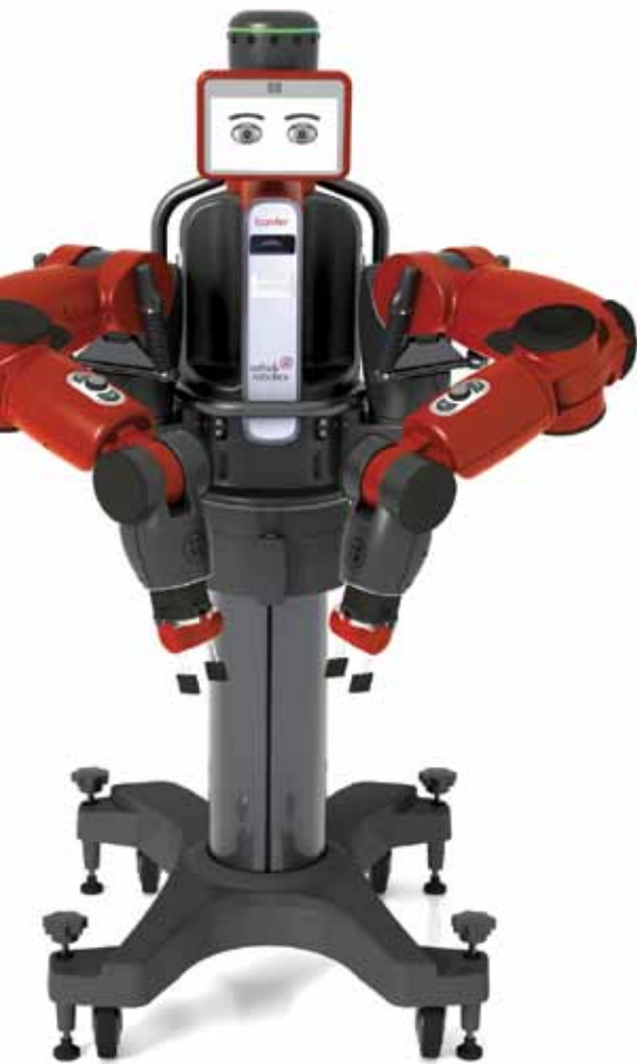
Baxter the Robot, from Rethink Robotics, is capable of sorting, loading, and light assembly.
